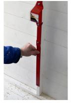
**15. Fit the side brace:** The last bolt will be fitted on the side brace, usually perpendicularly from the top extension bar. Another option would be with it fitted horizontally just above the floor, bolted to the bottom of the lower extension bar.
